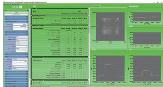
NR FDD sub-6 GHz Uplink TX Measurement using CombiView
