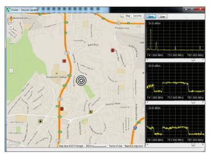
Figure 9. Geo-location of signal on map overlay
