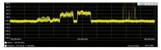
Figure 13. Trace Viewer display of all traces measured. *Notice intermittent signals on the right-hand side of trace.*
