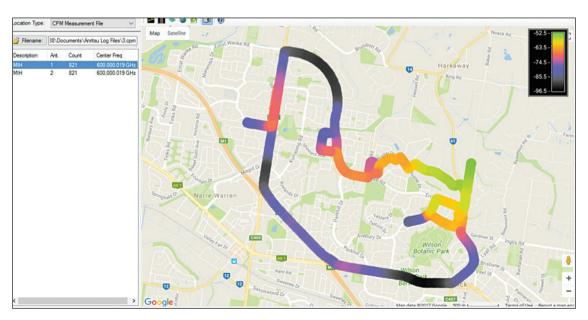
Figure 19. Coverage mapping display (Option 486)
